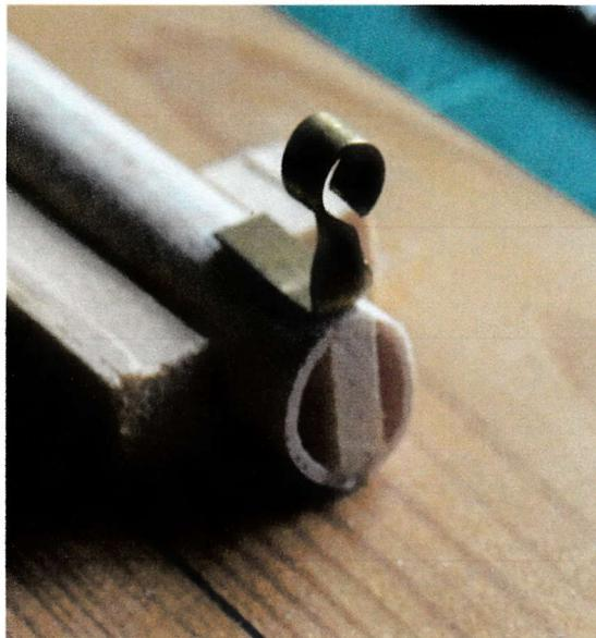
This method produces a strong prop hanger that can also be adjusted in any direction for thrust line changes. It is designed to hold a 'Peck' 1/32 Nylon bush, which fits snugly in the tube section.
